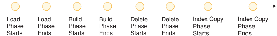
Figure 1. The Four Phases of the Load Process: Load, Build, Delete, and Index Copy. While the load operation is taking place, the target table is in the load in progress state. If the table has constraints, the table will also be in the check pending state. If the ALLOW READ ACCESS option was specified, the table will also be in the read access only state.
